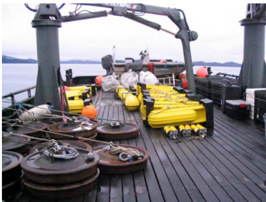
Vessel loaded with anchors and mooring equipment for initial deployment.
