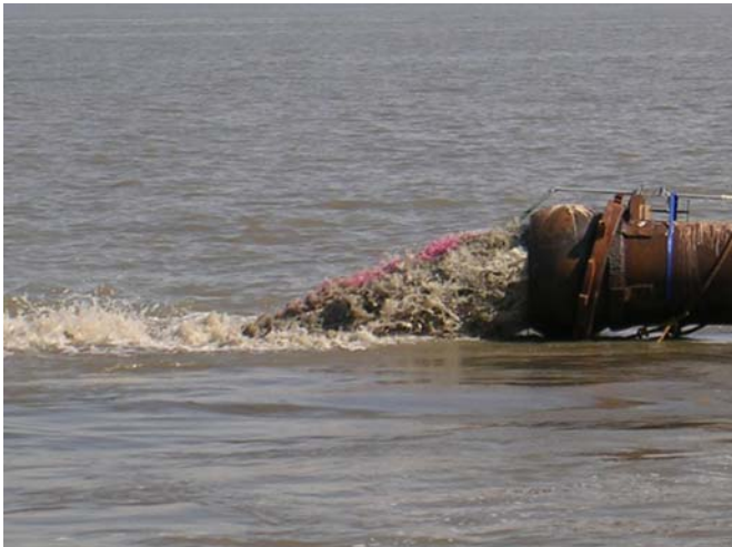
Tracer Being Injected into the Dredge Discharge
