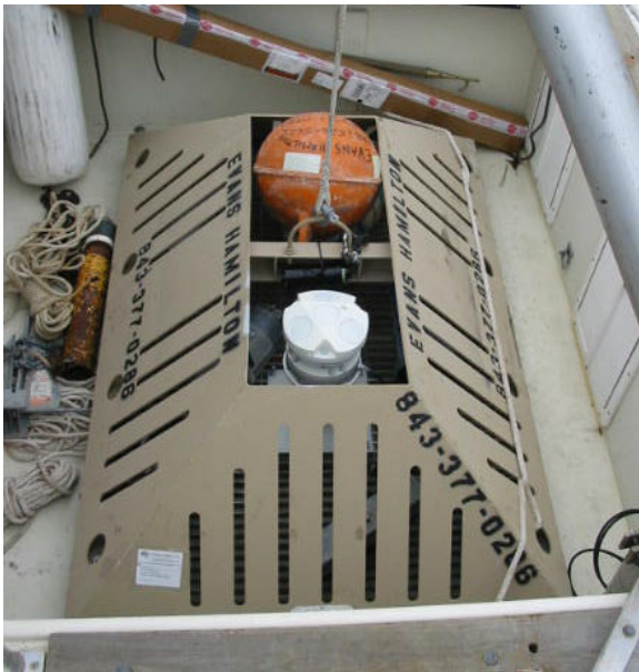
Instrument and Diverless Recovery System in Mount Prior to Deployment
