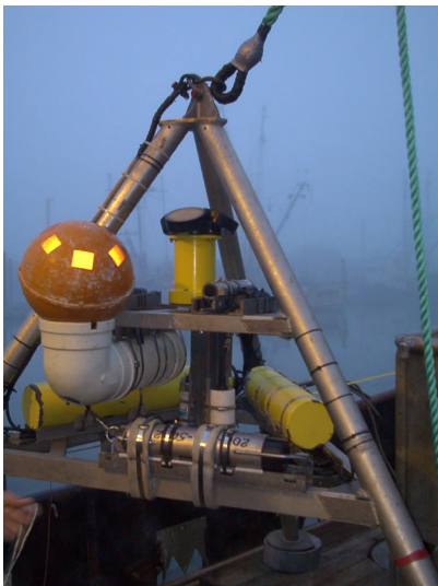
Oceanographic Tripod Instrumentation With ADCP and Acoustic Release.
