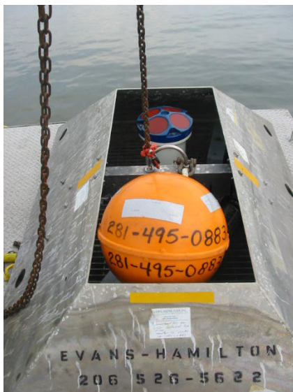
Bottom mounted ADCP in trawler-resistant pod.
